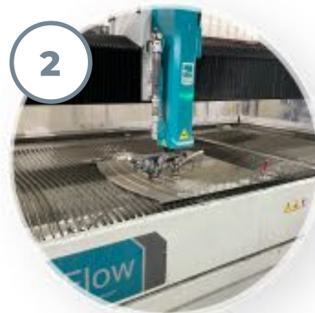
CNC WATER JET CUTTING
